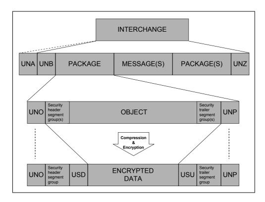
Figure 4 — Structure of an interchange containing one package whose contents (object and associated security header and trailer segment groups) have been encrypted (schematic)
