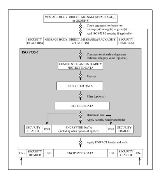
Figure B.1 — Processes involved in encryption of an EDIFACT structure
